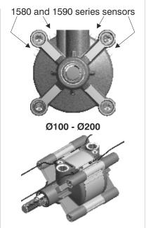
**CYLINDERS - BORE SIZE Ø100-Ø200:** All four housings can be accessed from the front of the unit. It is therefore possible to use both type of sensors: 1580 - 1590.
