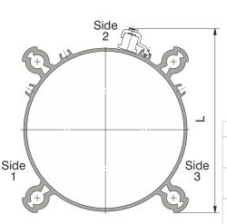
$\emptyset$ 125 -  $\emptyset$ 200: the sensors can be fixed on the three sides as indicated in the drawing, by using suitable bracket
