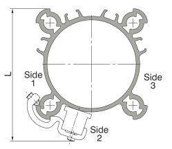
Ø32 - Ø100: the sensors can be fixed on the three sides as indicated in the drawing, by using suitable brackets (except for Ø32 on side 2)
