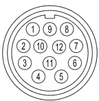
HA connector (12 pin) M23 CCW Hummel 7.410.000000 - 7.002.912.603 solder side view FV
