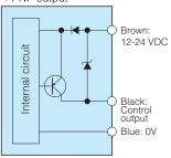
In the condition of load short circuit or overload, the output transistor turns off. Check the load condition before restarting.
