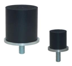
Material PUR, micro-cellular Base: steel, zinc plated Load 2 - 225 Nm Temperature -30°C - max. +80°C (-22°F - max. +176°F) Impcat speed max. 5 m/s Long life time Resistant to oil, grease, ozone, UV radiation, weathering and splash water **Applications** End stop of machines, Crane systems
