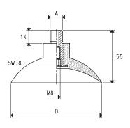
Note: The force of the vacuum cups indicated in the table represents 1/3 of the value of the theoretical force calculated at a level of vacuum of -75 KPa and a factor of safety 3. Transformation ratio: N (newton) = Kg x 9.81 (force of gravity) inch =  $\frac{mm}{25.4}$ ; pounds =  $\frac{g}{453.6}$  =  $\frac{Kg}{0.4536}$  Adapters for GAS - NPT threading available on page 1.130
