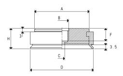
Note: The force of the vacuum cups indicated in the table represents 1/3 of the value of the theoretical force calculated at a level of vacuum of -75 KPa and a factor of safety 3. Transformation ratio: N (newton) = Kg x 9.81 (force of gravity) inch =  $\frac{mm}{25.4}$ ; pounds =  $\frac{g}{453.6}$  =  $\frac{Kg}{0.4536}$
